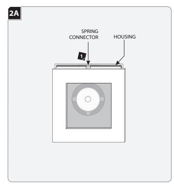
Align the trim spring connectors with the inner edge of the housing.
