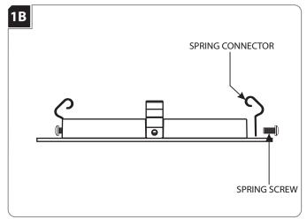
3 Replace the pre-installed spring connectors by removing the spring screws.
