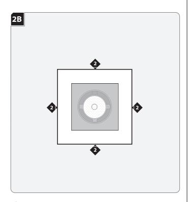
2 Gently push the trim into the housing so that the four spring connectors snap into place.
